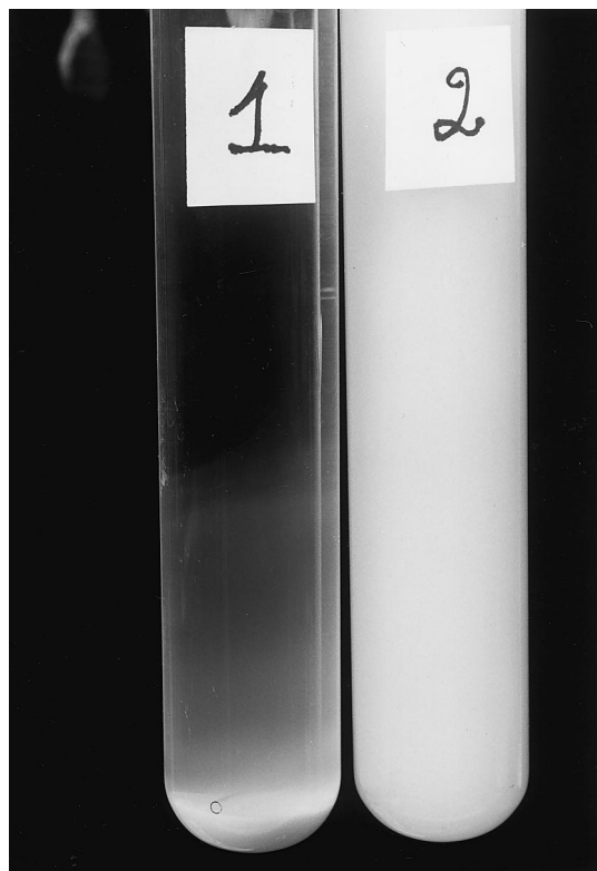
Figure 1. Addition of 0.015% hesperidin solution, previously solubilized in NaOH, to: 1) 0.2% commercial pectin, of which the particles flocculate on the bottom of the tube; 2) 0.2% commercial pectin, of which formed stable colloidal particles in the solution.
